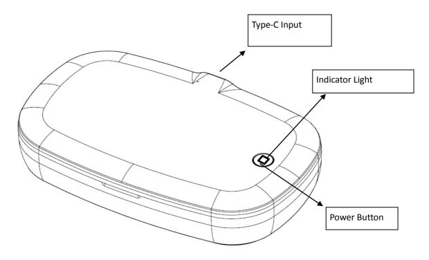
There is no lithium battery inside this product. It is powered by the Type-C cable connecting to the power source.
