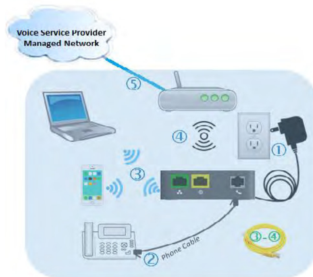
Figure 3. Setup the MTA device to connect to the router or network switch
