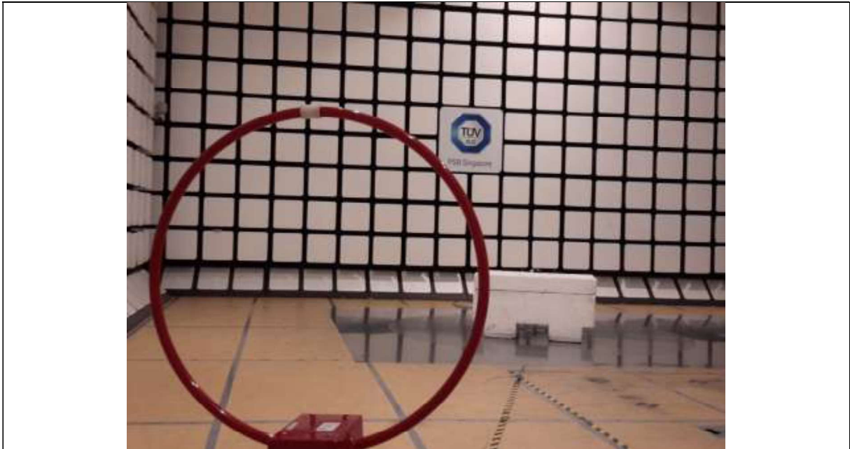
Radiated Emissions (Spurious Emissions Inclusive Restricted Bands Requirement) Test Setup (Front View)
