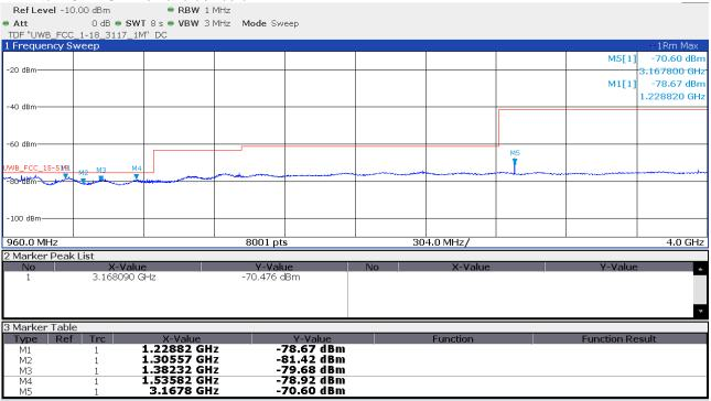
Note: The emission points M1 – M5 are not a result of UWB transmission but of the device itself. They comply with the general limit of §15.209.
