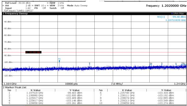
Note: The emission point M1 is not a result of UWB transmission but of the device itself. It complies with the general limit of §15.209.
