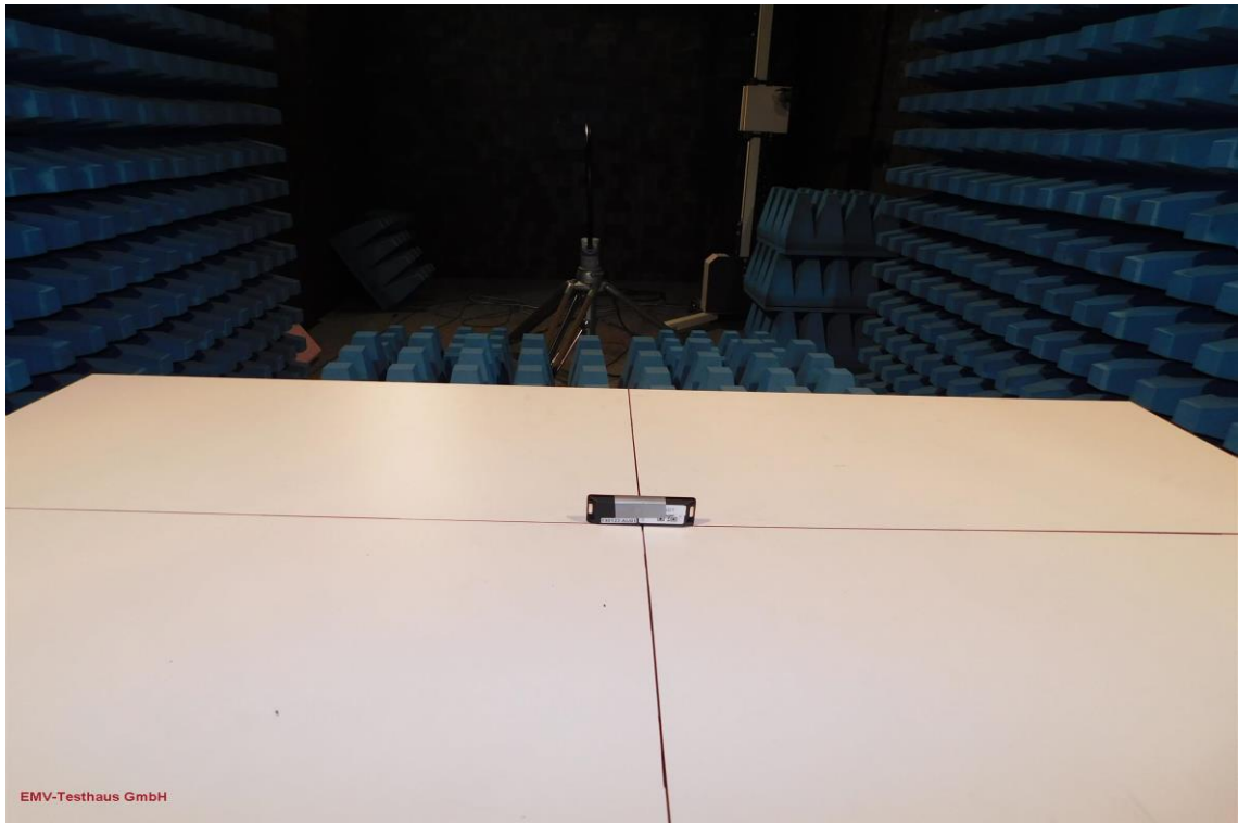
Picture 11: EUT test setup radiated emissions test from 9 kHz to 30 MHz
