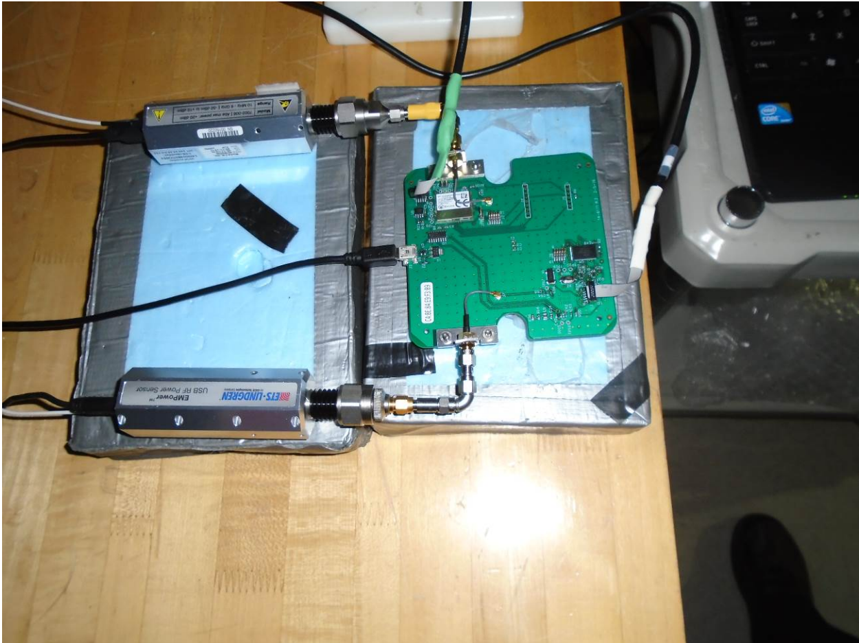
Figure 5: Close-up view of Conducted RF Emissions Test Setup for Co-Location Power test setup
