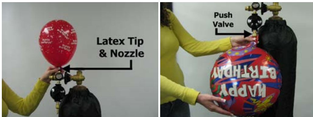
Figure 20: (Left) Latex Balloon Inflation, (Right) Foil Balloon Inflation
