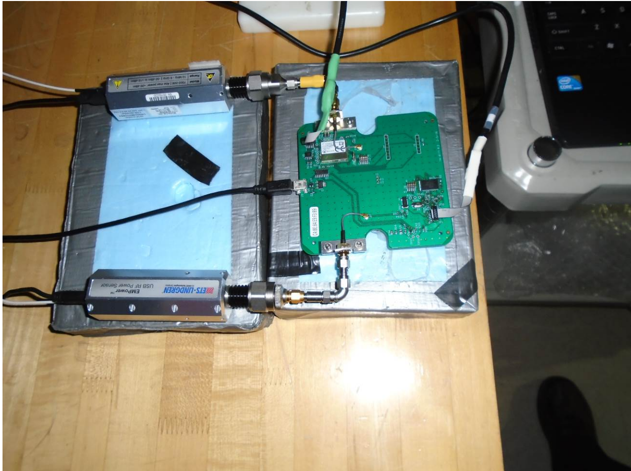
Figure 13: Close-up view of Conducted RF Emissions Test Setup for Co-Location Power test setup
