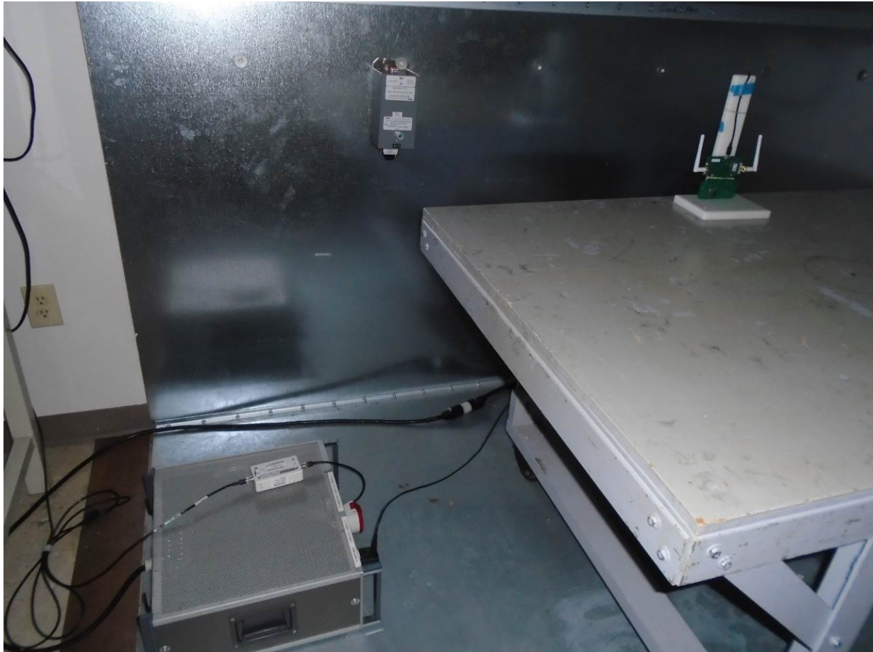
Figure 9: Conducted Emissions on AC Mains Test Setup
