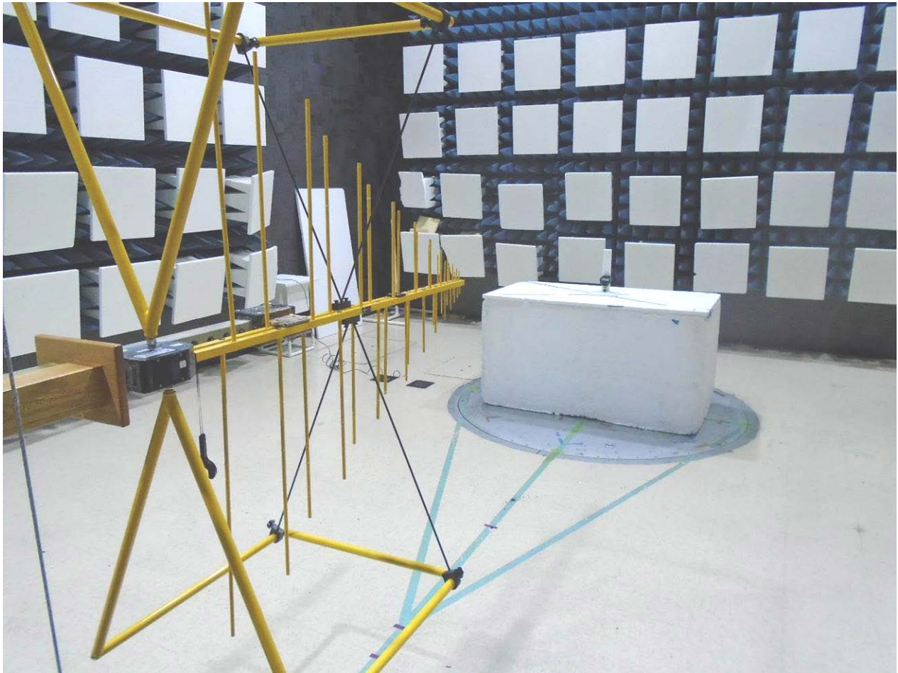
Figure 1: Typical Radiated Emissions – 30 MHz to 1 GHz shown, Front view Orientation “A” shown
