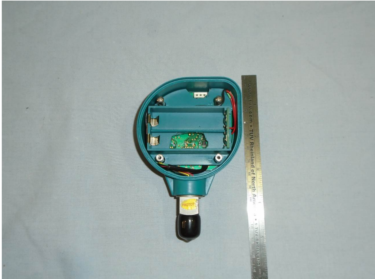
Figure 2: View of Modified EUT to allow programming the transmitter without removing batteries.
