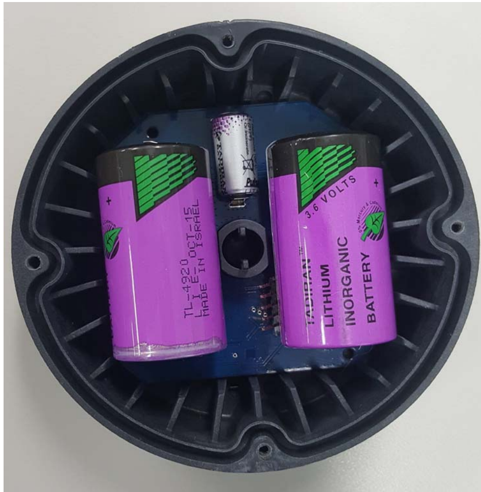
Top of PCB inside case with batteries and capacitor
