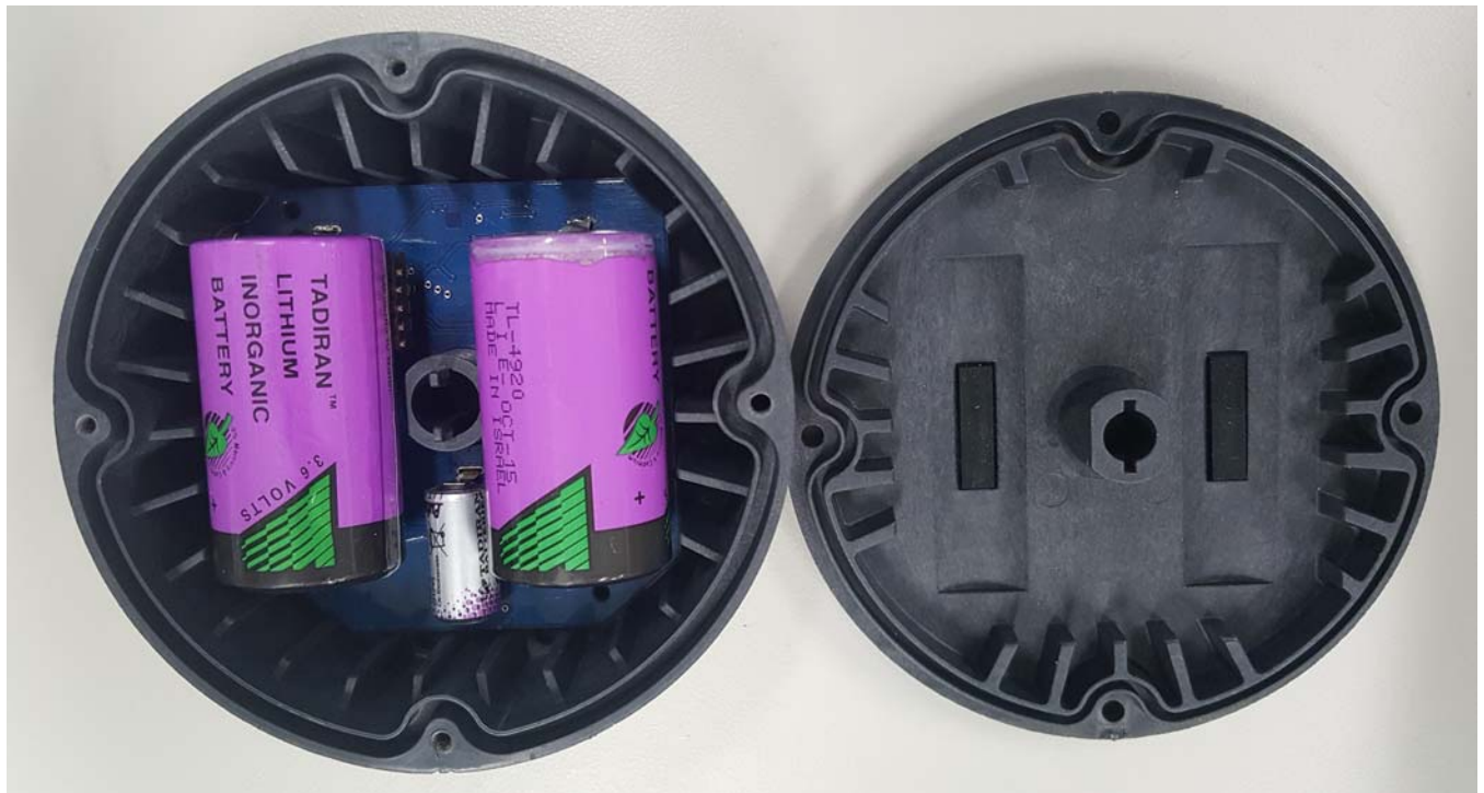
Top of PCB inside case with batteries and capacitor
