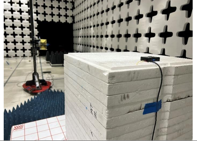
Radiated Emission Test above 1GHz Rear View
