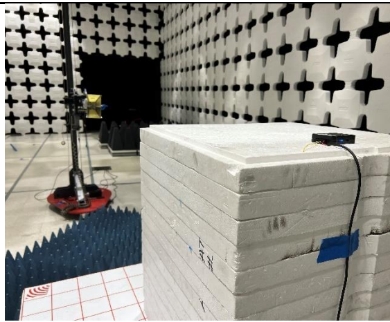
Radiated Emission Test below 1GHz Rear View
