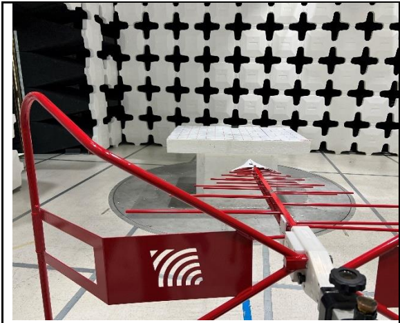
Radiated Emission Test below 1GHz Front View
