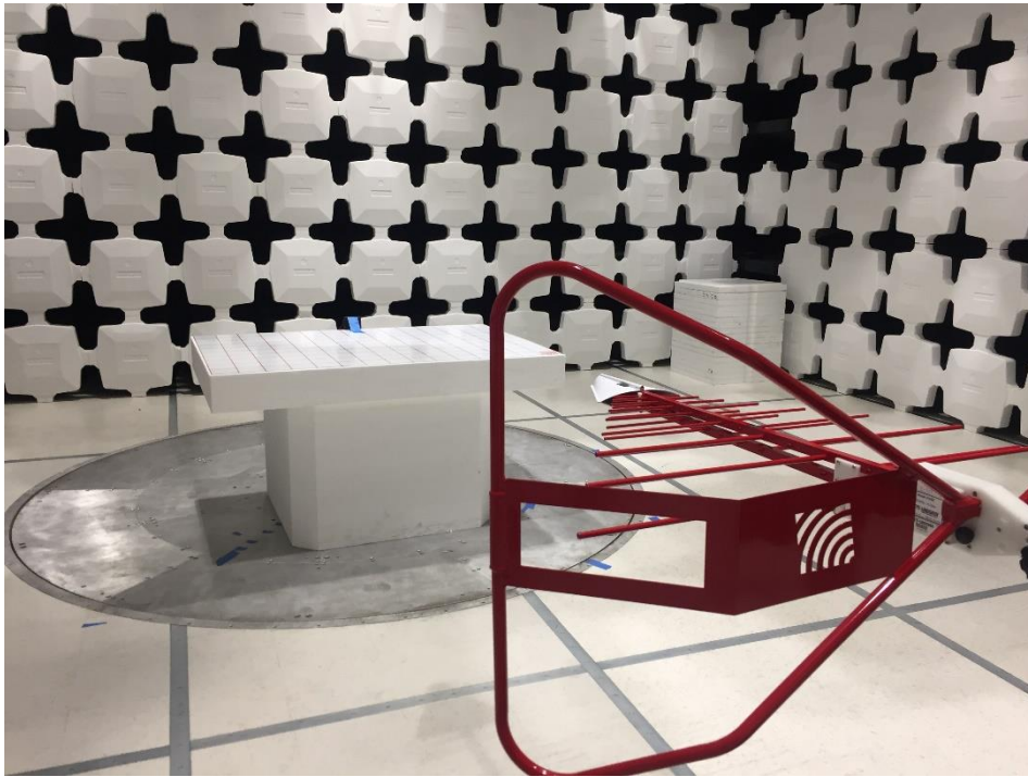
Radiated Emissions Below 1GHz setup – Front
