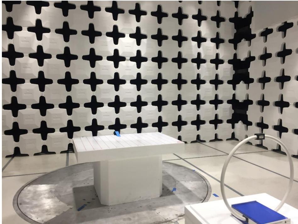
Radiated Emissions Below 30MHz setup – Front
