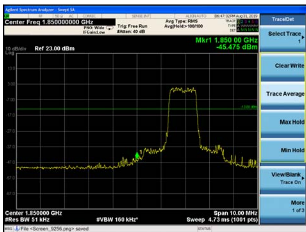
LTE Band 25 20MHz QPSK 100%RB CH-Low
