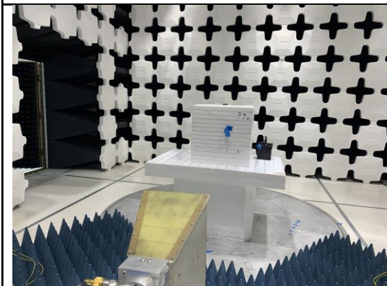
Radiated Emission Test above 1GHz Front View
