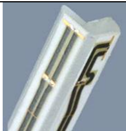
Fig 5.2 Photo of E-field Probe
