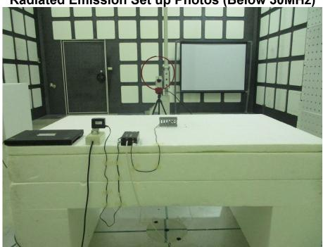
Radiated Emission Set up Photos (Below 1GHz)
