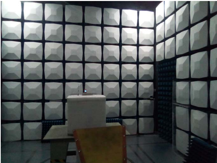
Radiated Emission View (Above 1GHz)
