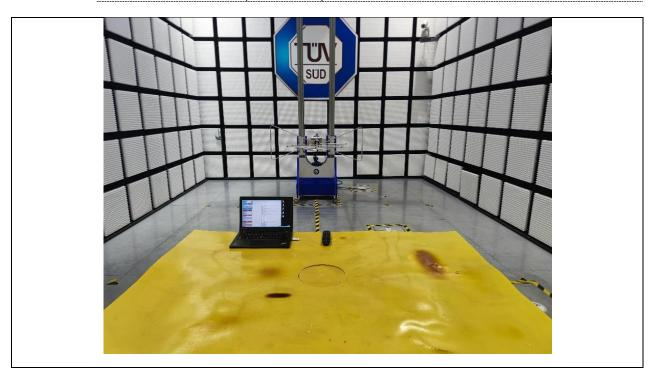
Details of: Radiated Emission test (1-18GHz)
