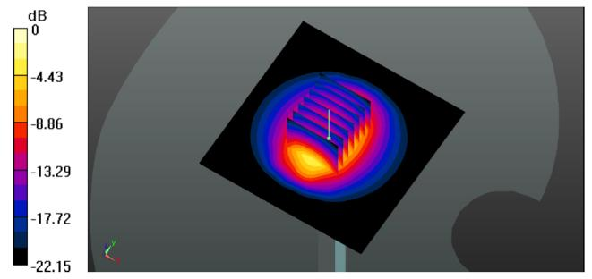
System Performance Check 2450MHz Body250mW
