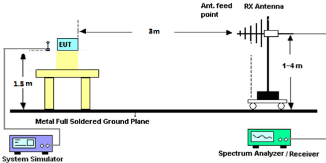
For radiated test from above 1GHz
