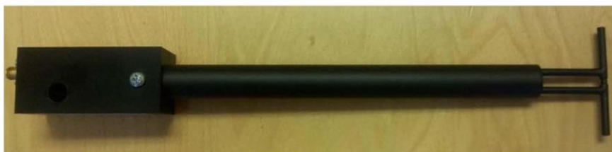
Figure 1 – MVG COMOSAR Validation Dipole
