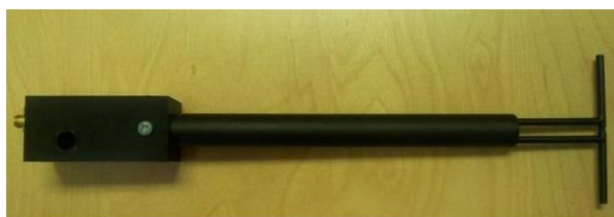
Figure 1 – MVG COMOSAR Validation Dipole
