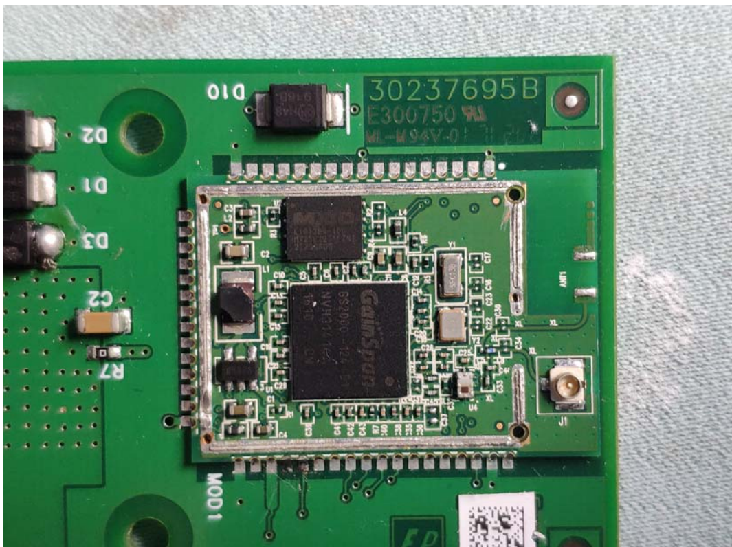
FIGURE 18 WEIGHING TERMINAL (M/N: IND256X) CRYSTAL & CHIP ON RF BOARD
