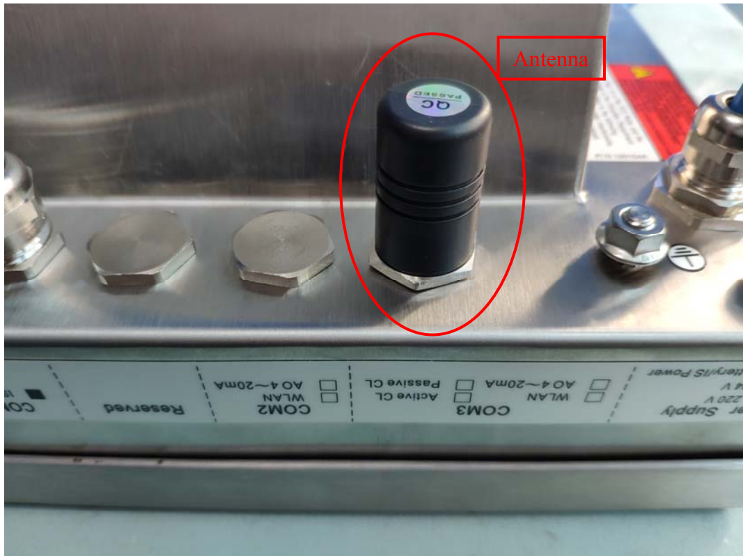
FIGURE 8 WEIGHING TERMINAL (M/N: IND256x) ANTENNA
