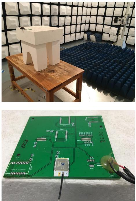
Test Setup For Radiated Emission (Above 1GHz)
