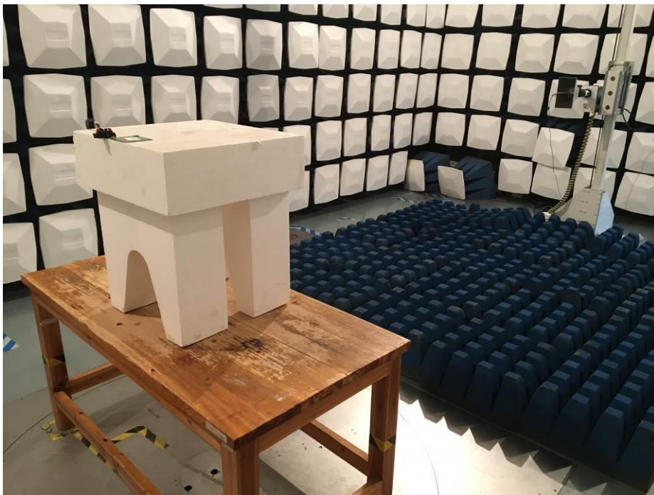
Test Setup For Radiated Emission (Above 1GHz)
