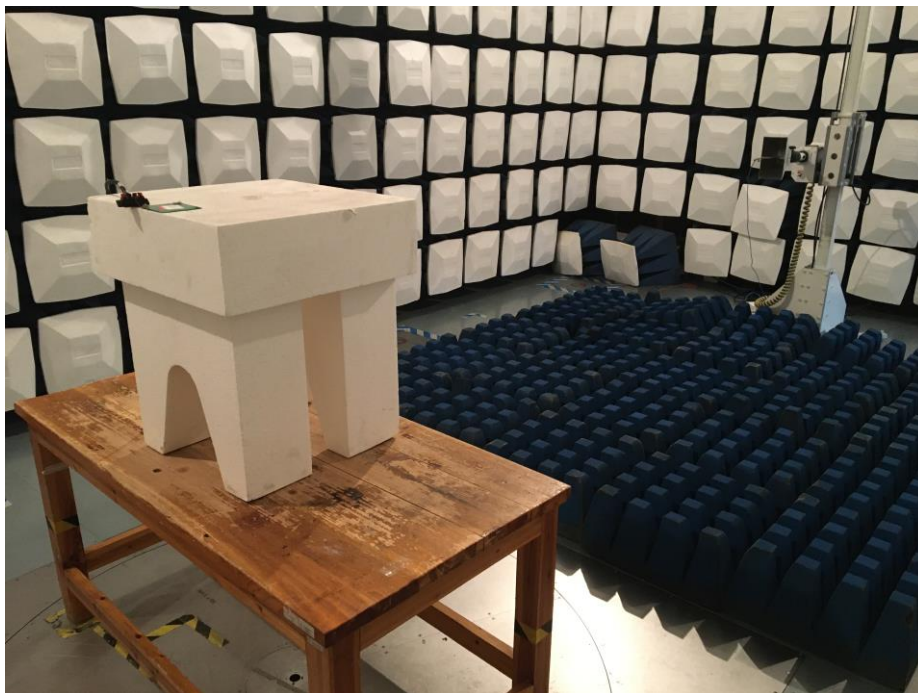
Test Setup For Radiated Emission (Above 1GHz)
