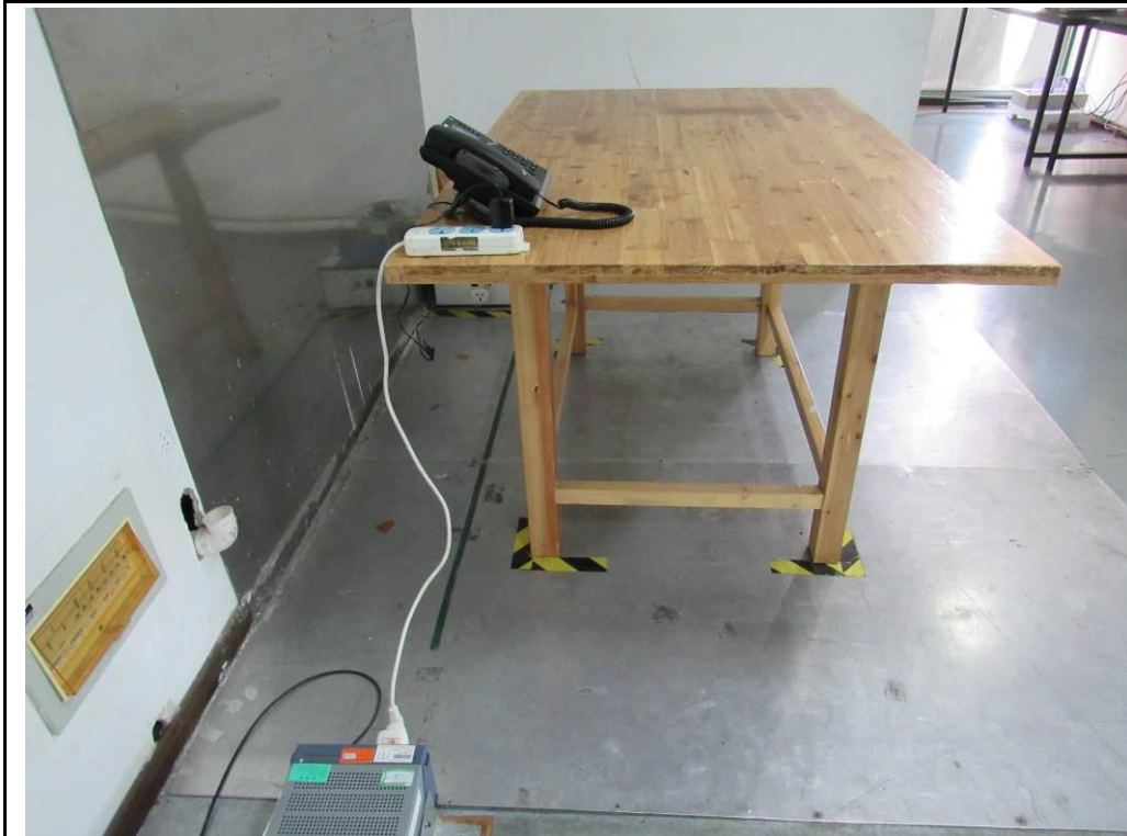
Conducted Emissions Test Setup Side View
