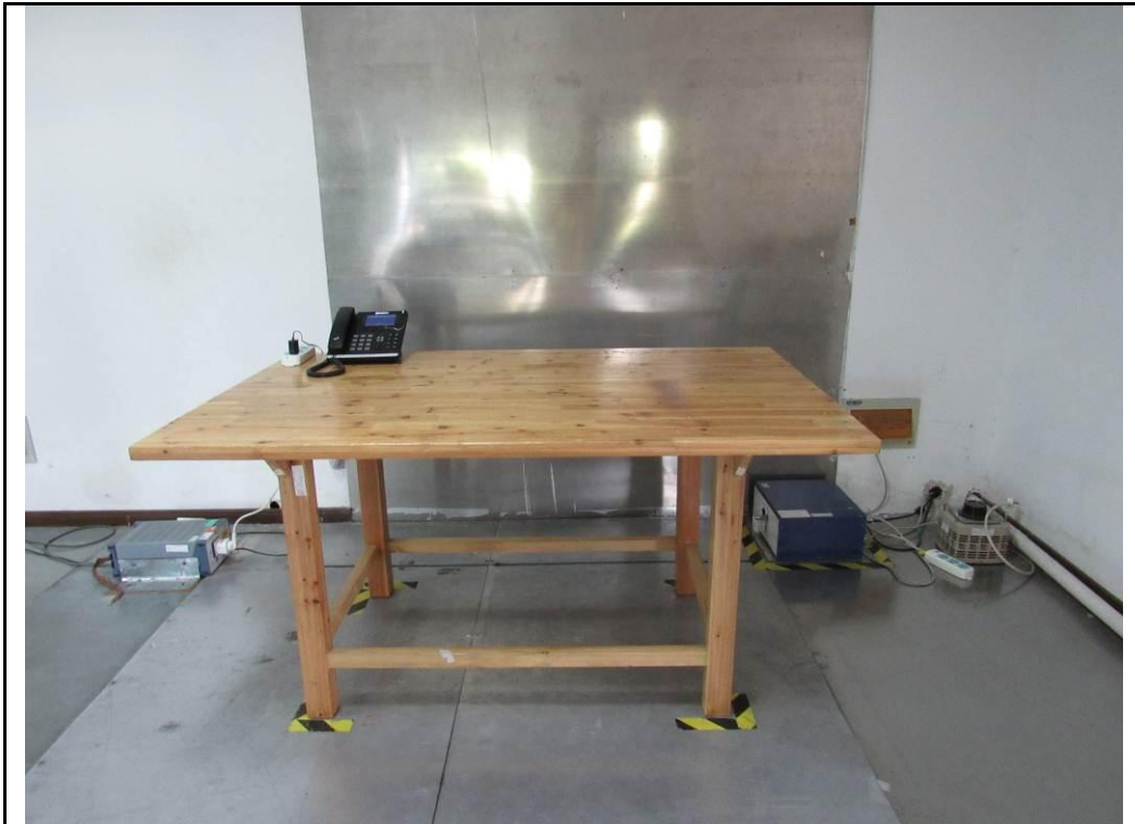
Conducted Emissions Test Setup Front View
