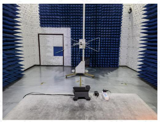
RADIATED EMISSION TEST SETUP ABOVE 1GHz
