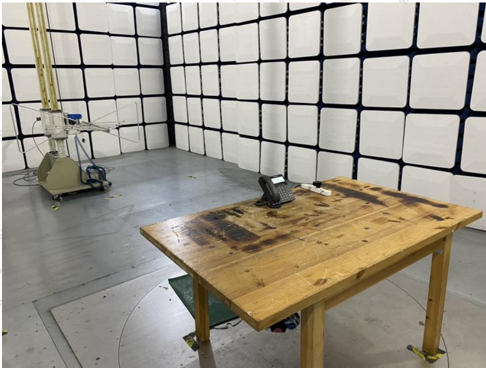
Photo of Radiation Emission Test
