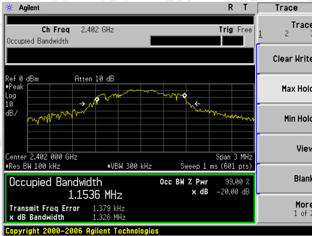
TEST PLOT OF BANDWIDTH FOR LOW CHANNEL
