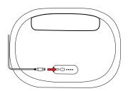
Insert the other end of the USB cable into a suitable USB charging adapter.
