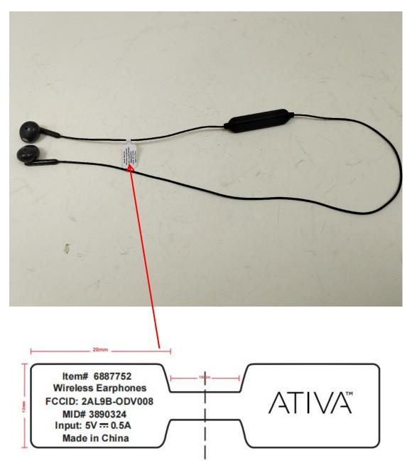
The nameplate is made of tough material, which is not easy to be damaged, and it is stuck on the earphone cable of the product. The earphone cable and the wireless part are integrated and cannot be separated.
