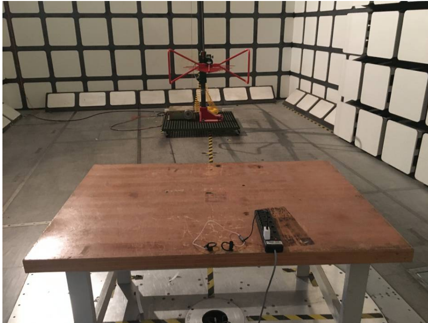
Radiated Emissions – Front View (Below 1 GHz)
