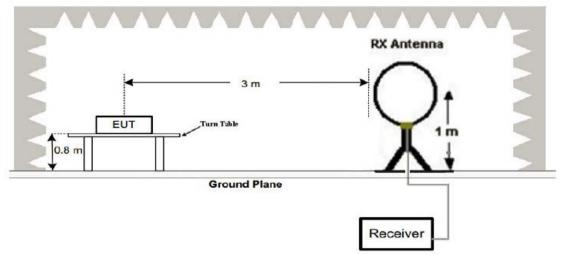
(2) Radiated Emission Test-Up Frequency 30MHz~1GHz
