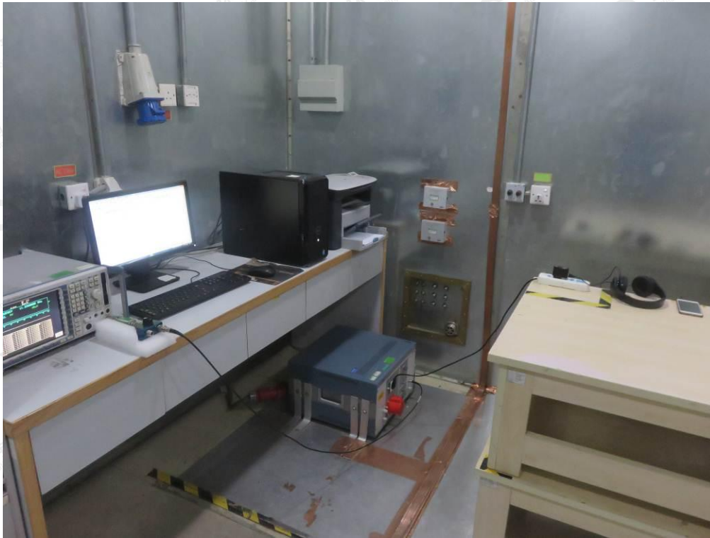
FCC RADIATED EMISSION TEST SETUP
