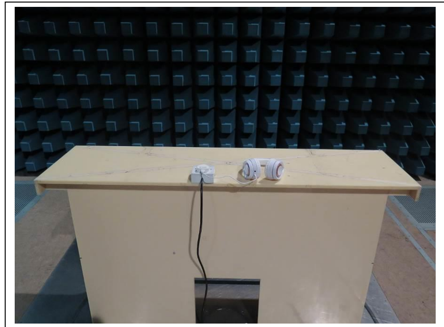
Charging (for radiated)
