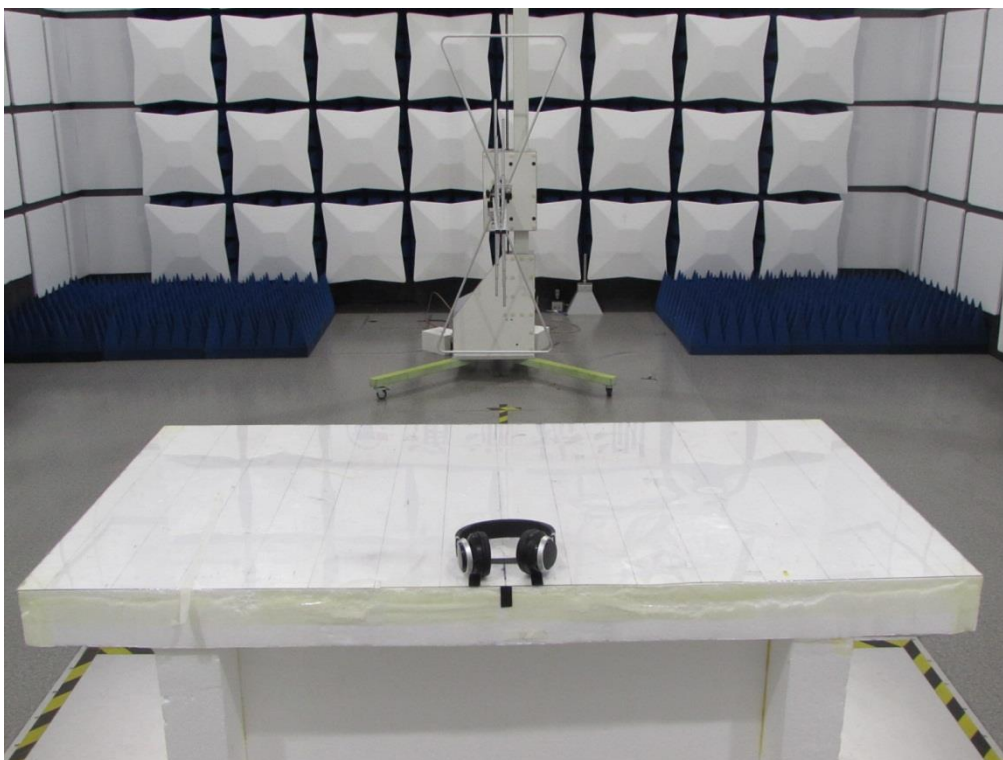
Radiated Emission Above 1GHz
