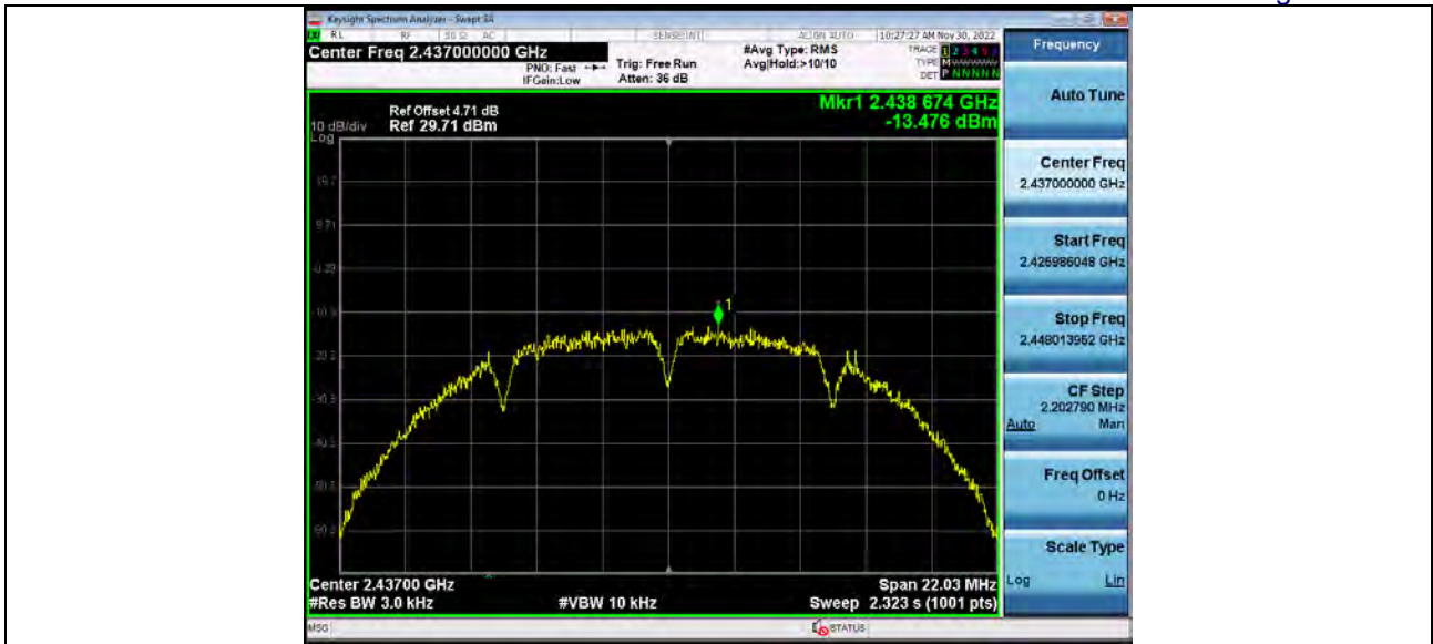
Power Spectral Density 2_4GWiFi_802_11b_2462
