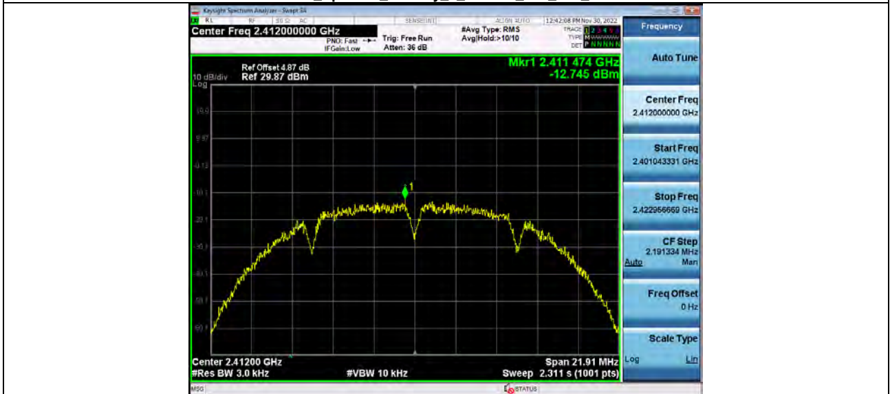
Power Spectral Density 2_4GWiFi_802_11b_2412
