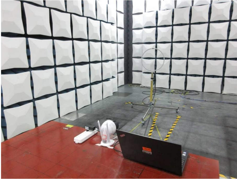
RADIATED RF MEASUREMENT SETUP (9KHz ~ 30 MHz)
