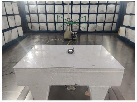
Radiated Emissions (9kHz-30MHz)
