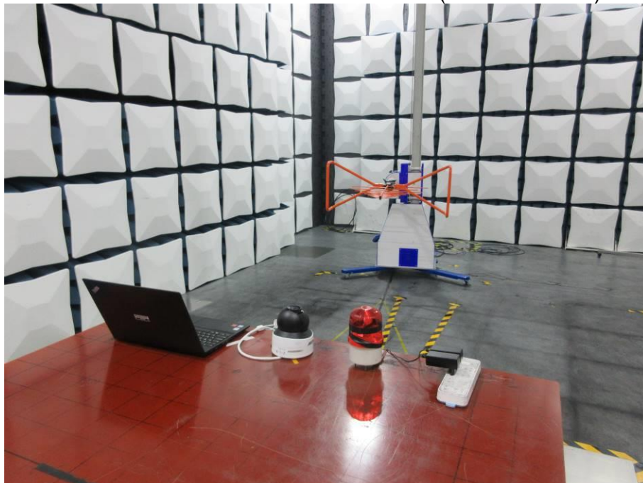
RADIATED RF MEASUREMENT SETUP (30MHz ~ 1 GHz)
