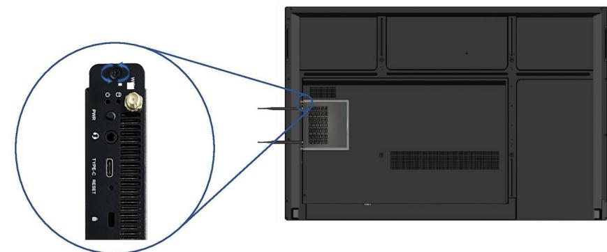
**Step 5:** Press the small Power Button on the back of the OPS to power it on. It can also be powered on from the 'Source' option in your OneScreen Panel.
