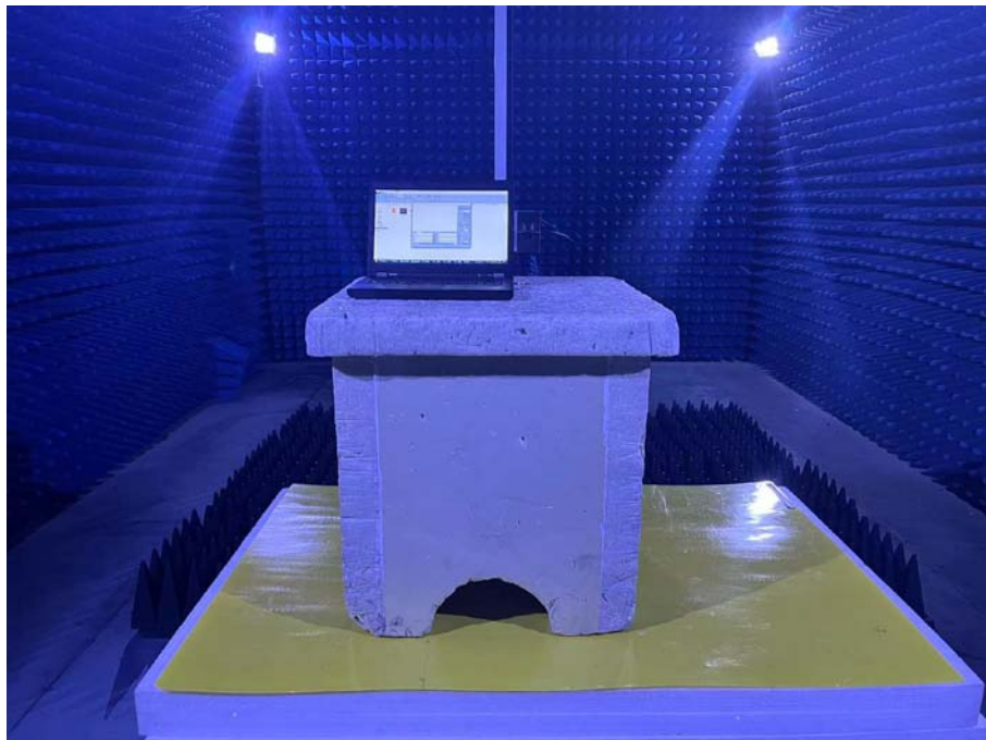
Photo of Radiated Emission Measurement Above 1GHz
