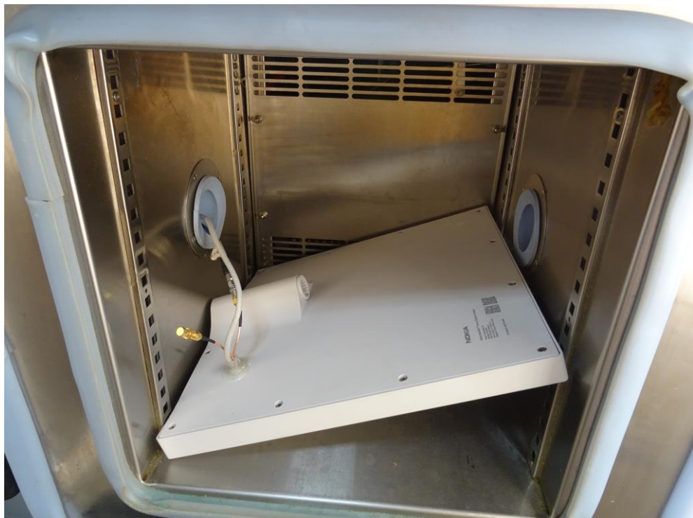
Antenna Port Measurement Test Setup – Thermal Chamber
