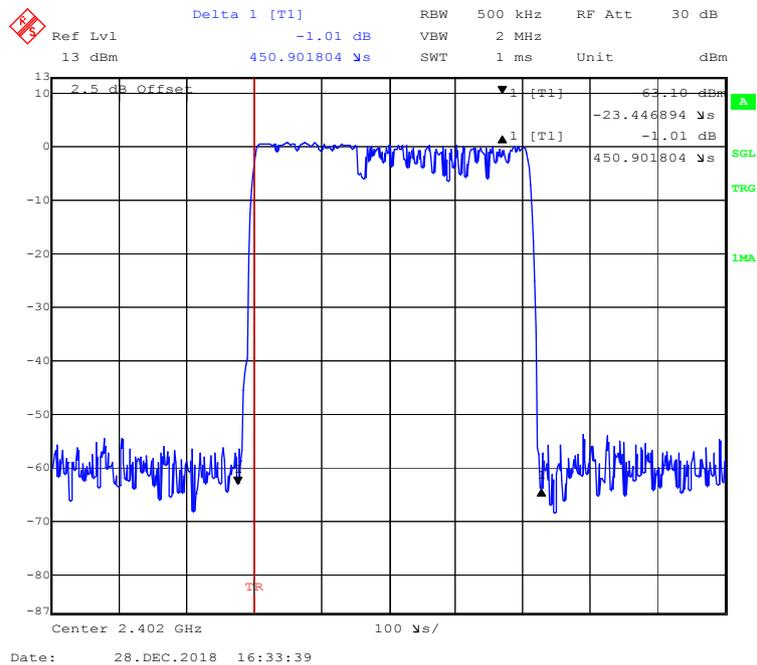
**EDR (8DPSK): Pulse time, Middle Channel, 3DH1**
