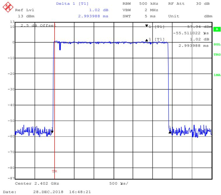
**EDR (8DPSK): Pulse time, Middle Channel, 3DH5**
