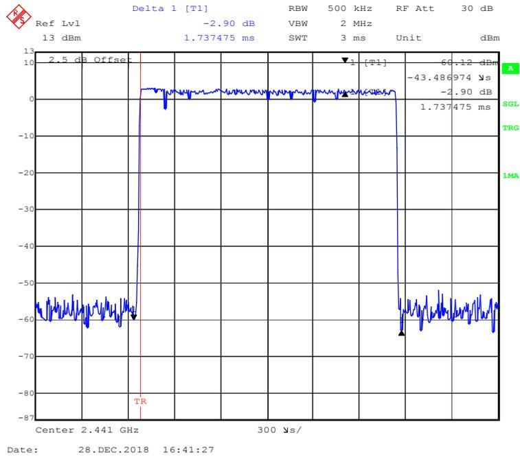
**EDR (8DPSK): Pulse time, High Channel, 3DH3**
