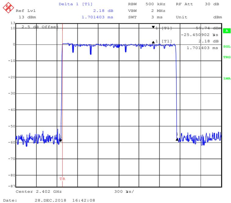
**EDR (8DPSK): Pulse time, Middle Channel, 3DH3**
