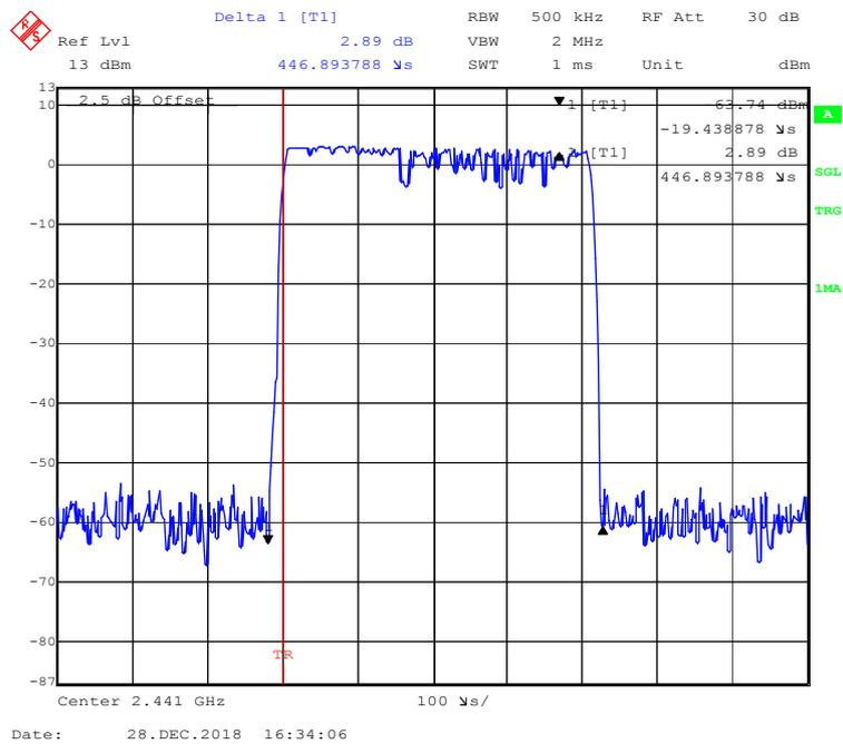
**EDR (8DPSK): Pulse time, High Channel, 3DH1**
