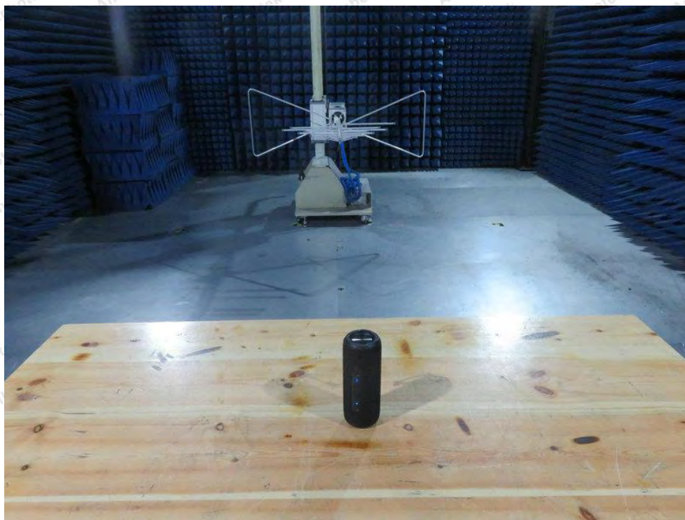
Photo of Radiation Emission Test
