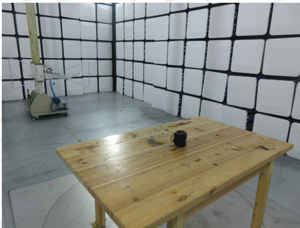
Photo of Radiation Emission Test
