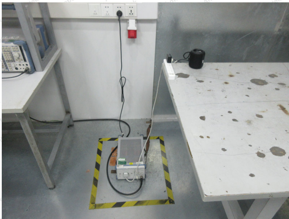
Photo of Conducted Emission Measurement
