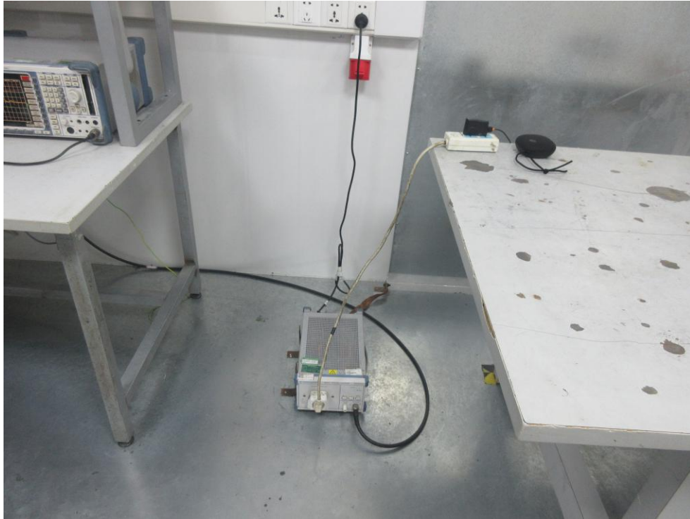
Photo of Conducted Emission Measurement
