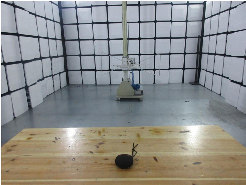
Photo of Radiation Emission Test
